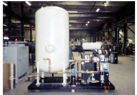
Tate Engineering/ZBZ & Associated, Inc./Sea Tack Community Center, Virginia Beach, VA skid-mounted WH1210 with storage tank for domestic hot water & building heat (providing combination service).
