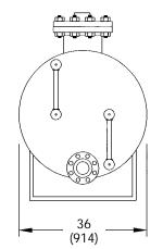
Exhaust outlet: 2" NPT Motive inlet: 2" NPT
