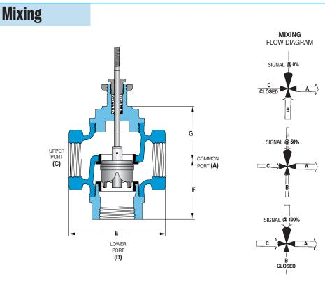
Trerice 3-Way Valves are not designed for use in steam applications. To properly control the mixing of two flows, inlet pressures at ports B and C should be as equal as possible.
