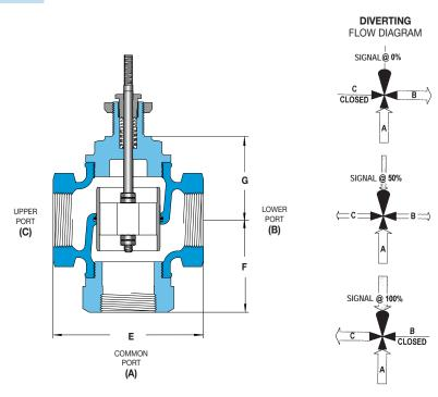
Trerice 3-Way Valves are not designed for use in steam applications.
