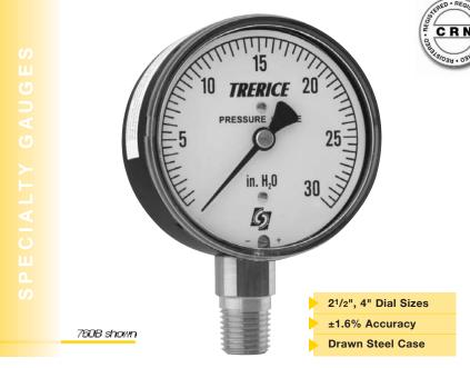
The Trerice **760B** Low Pressure Gauge is designed to accurately measure extreme low pressure conditions. This pressure gauge employs a diaphragm capsule sensing element to measure the low pressure. Case material is drawn steel with brass wetted parts. Optional features and case style variations available: Please consult the Options & Accessories Section for details.
