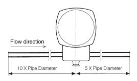
To function properly, all models of the KEL require lengths of straight piping to be plumbed into the units at the inlet and outlet fittings. The inlet length must be 10 times the pipe diameter. The outlet length must be 5 times the pipe diameter.
