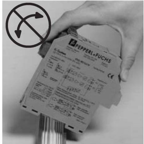
INCORRECT: Unit snapped on at an angle
